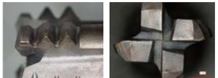
Epoch D Thread Mill after threading 50 holes.
