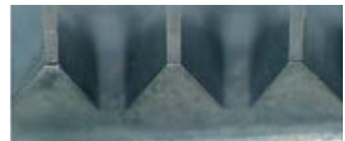
Epoch Thread Mill after threading 300 holes.
