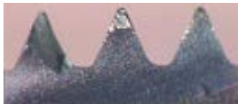
Conventional after threading 10 holes.
