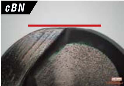
先端部の摩滅が大きい Significant tip wear
